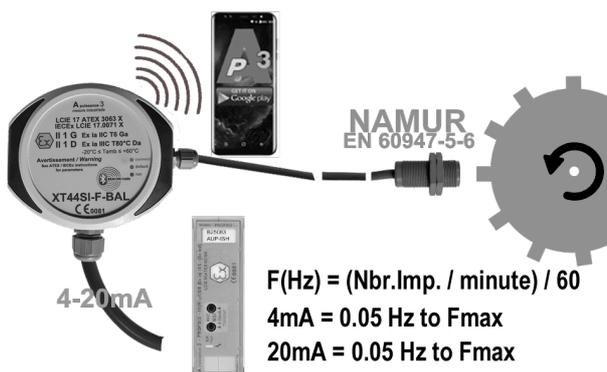
$F(\text{Hz}) = (\text{Nbr. Imp.} / \text{minute}) / 60$
