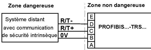
**Raccordement de la fonction communication + alimentation**
